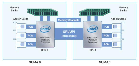
Each physical CPU and attached resources including memory and connected PCIe buses are grouped by a NUMA address. Each NUMA is interconnected with a dedicated point-to-point communications technology. The Intel version is called QuickPath Interconnect (QPI). In 2017, Intel released the Ultra Path Interconnect (UPI), replacing QPI.
