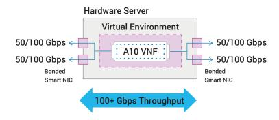
Figure 5: VNF high-performance platform (bonded NIC ports)
