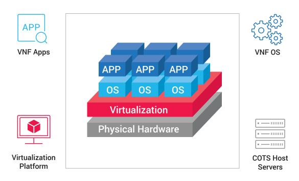
Figure 3: VNF server platform functional layers
