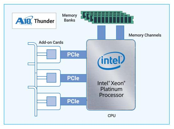
Figure 10: Simplified server architecture components
