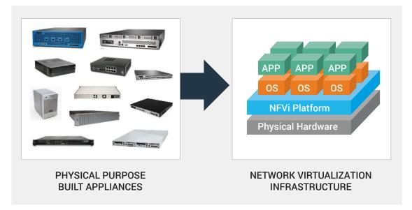
Figure 1: Transformation of specialized hardware to virtualization platforms
